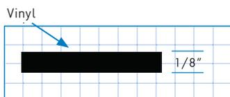
Specially treated for flooring applications, this non-conductive matting meets **Mil. Spec. 15562-G, Type I**.
